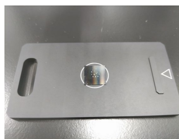
Fig. 2 Si Filter Installed in the PF Holder
