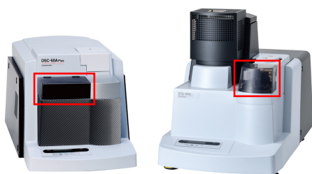
Fig. 1 Appearance of (Left) DSC-60A Plus and (Right) DTG-60A (The red boxes show the autosamplers.)
