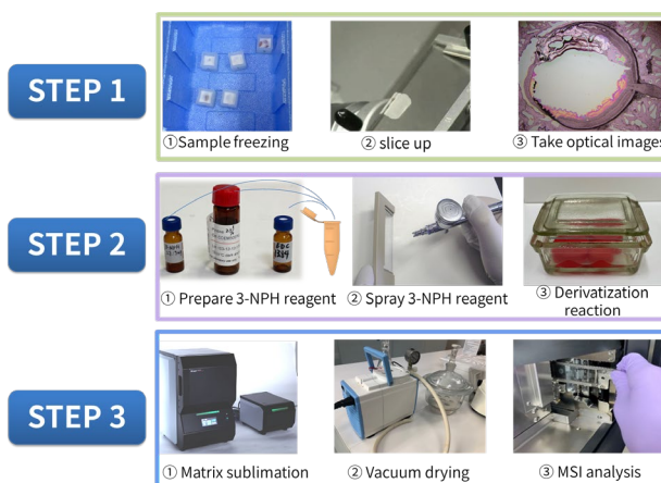
Figure 2 mouse eyeball slice derivatization flow chart
