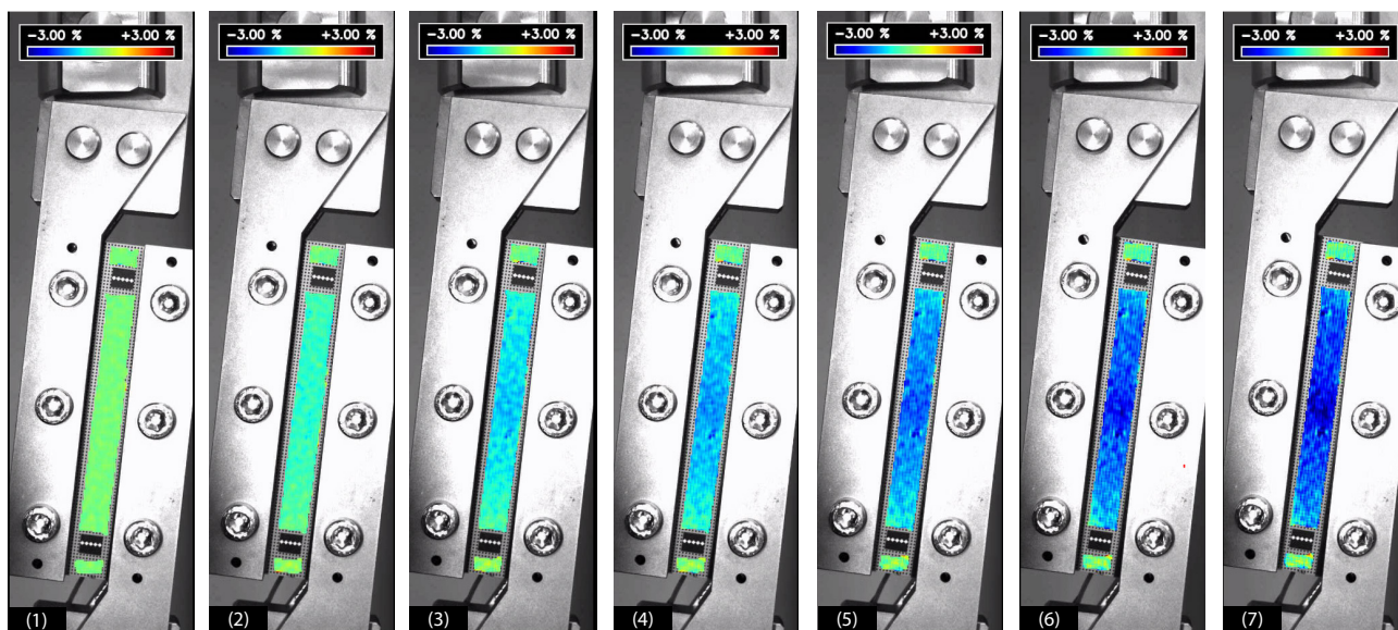
Fig. 6 Shear Strain Distribution by Real-Time Strain View *The direction of shear strain is the opposite of the definition in the standard.
