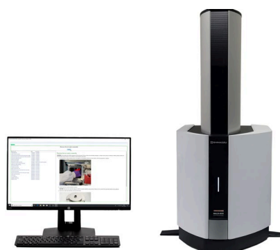
Figure 1. Shimadzu MALDI-8030 EasyCare MALDI-TOF mass spectrometer.
