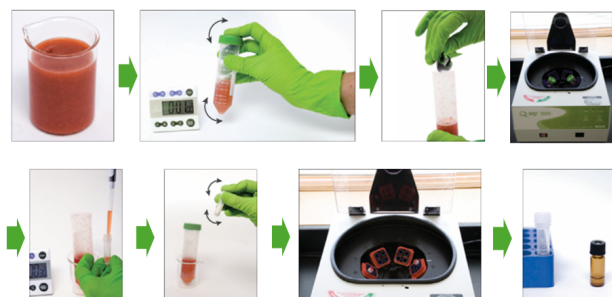
Fig. 5 Example of Sample Preparation Using QuEChERS
