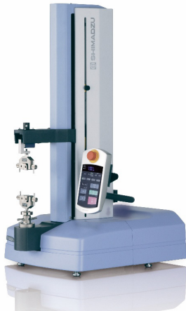
Fig. 1 Appearance of EZTest Texture Analyzer
