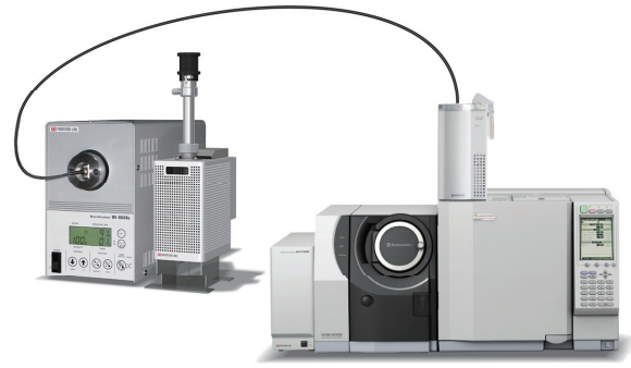
Fig. 2 UV-Py/GC-MS system (UV-1047Xe+PY-3030D+GCMS-QP2020)
