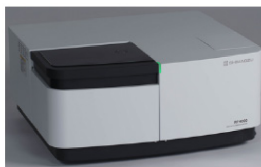
Fig. 1 Shimadzu spectrofluorophotometer, RF-6000, used for fluorescence measurements
