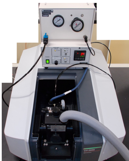
Fig. 1 Condition of CoolSpeK Attached to UV-2600
