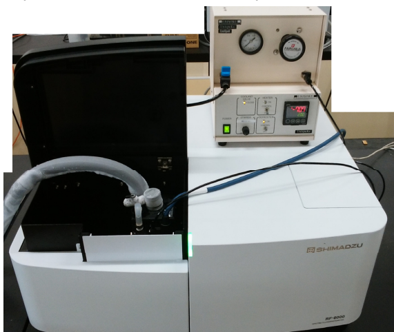
Fig. 4 Condition of CoolSpeK Attached to RF-6000
