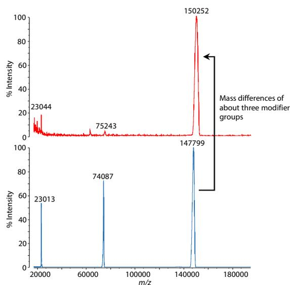
Fig. 3 Mass Spectra of Modified Antibody (top) and Untreated Antibody (bottom) Antibody
