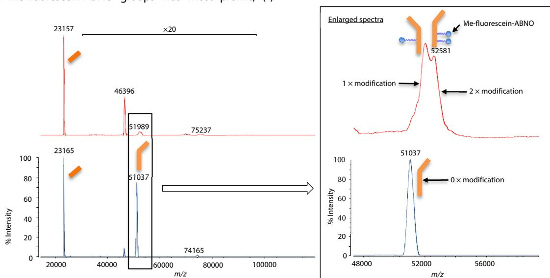
Fig. 4 Mass Spectra of Modified Antibody (top) and Untreated Antibody (bottom) After Reduction Treatment
