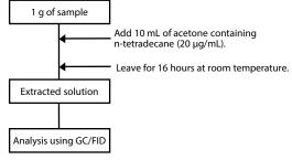
Fig. 2 Pretreatment Method for Silicone Products
