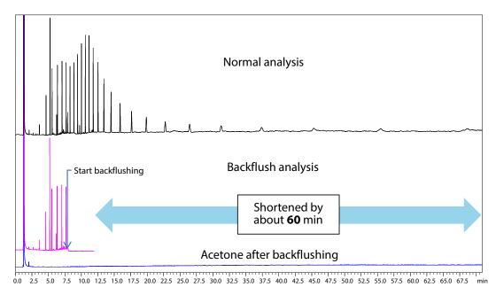
Fig. 3 Comparison of Chromatograms Obtained by GC/FID
