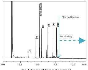
Fig. 4 Enlarged Chromatogram of Measurement with Backflushing
