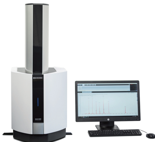
Fig. 1 Appearance of Benchtop MALDI-TOF MS "MALDI-8020"
