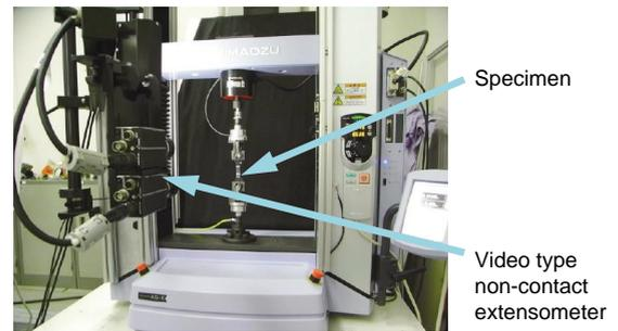
Fig. 5 Specimen and Extensometer
