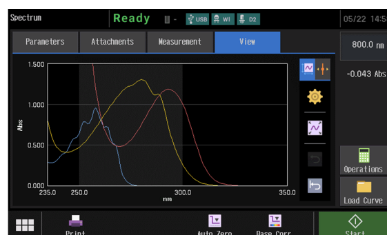
Fig. 7 Absorption Spectra Blue: Tyrosine (0.01 mol/L), Yellow: Tryptophan (0.005 mol/L), Red: phenylalanine (0.1 mol/L)
