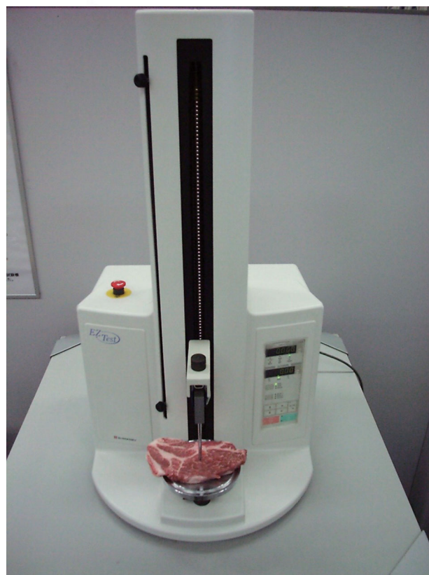
Fig. 2 Penetrating Strength Test Being Performed on Pork
