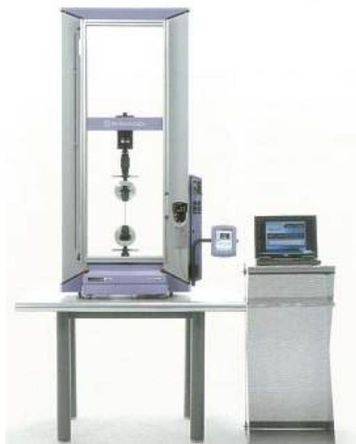
AG-Xplus Table-Top Precision Universal Tester
