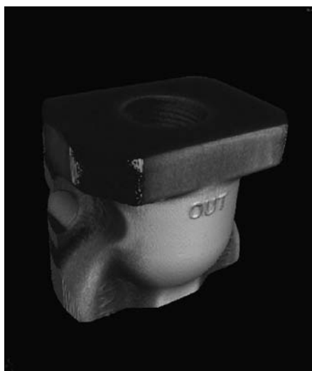
Fig.5 Example of 3-Dimensional Image for an Aluminum Die Cast Part
