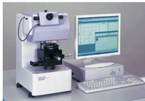
Fig. 1 Overview of Shimadzu DUH-211S Dynamic Ultra Micro Hardness Tester
