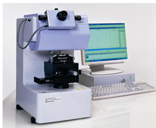
Fig. 2 SHIMADZU DUH-211 Dynamic Ultra-micro Hardness Tester
