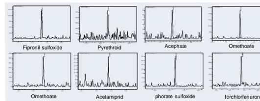
Figure 7 EIC of 0.1 ng/mL Partial Pesticide Mixed Standard
