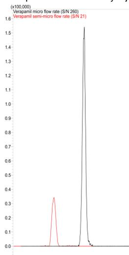
Subsequently the plug and play micro ESI ion source was substituted with ESI source and the Mikros Pump was used at semi micro flow rates for repeating the same analysis in semi-micro conditions (table 3, conditions comparison). Increase of signal intensity when using micro-flow rates system was >4.5 fold (>10 fold in S/N) for Verapamil and >3.5 fold for NorVerapamil (Figure 2).
