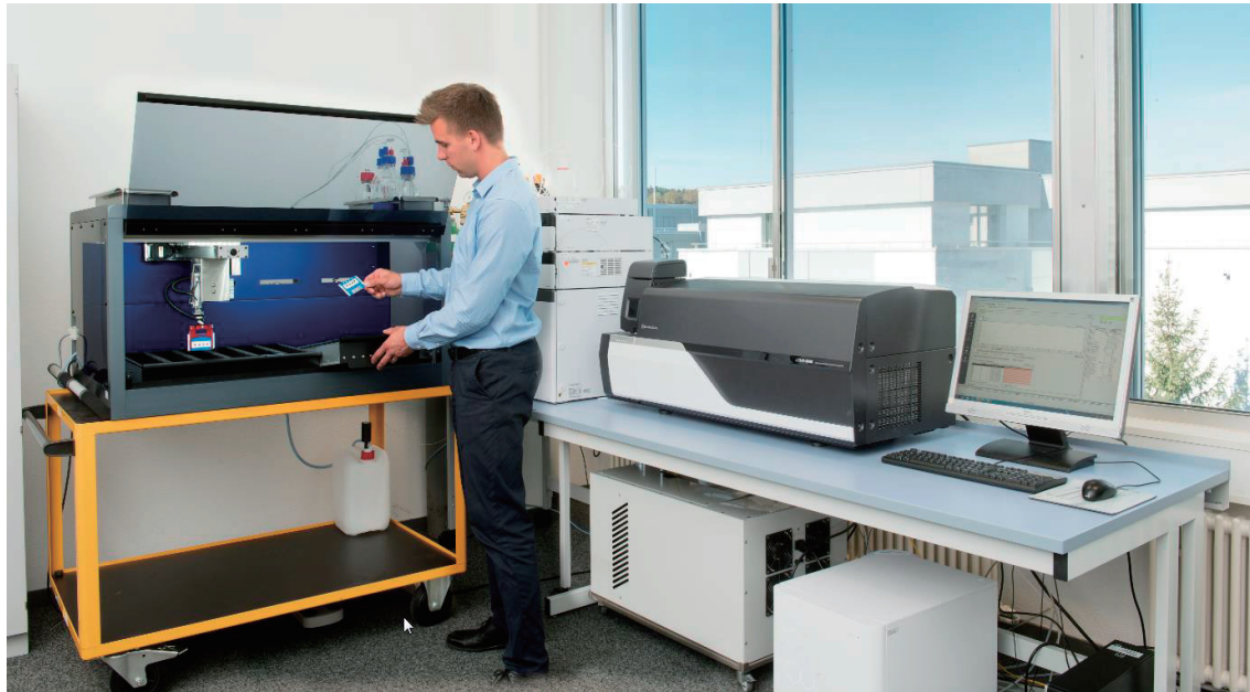
Figure 1 Instrumental setup: DBS-MS 500 (CAMAG, Switzerland), Nexera X2 UHPLC (Shimadzu, Japan), LCMS-8060 (Shimadzu, Japan)
