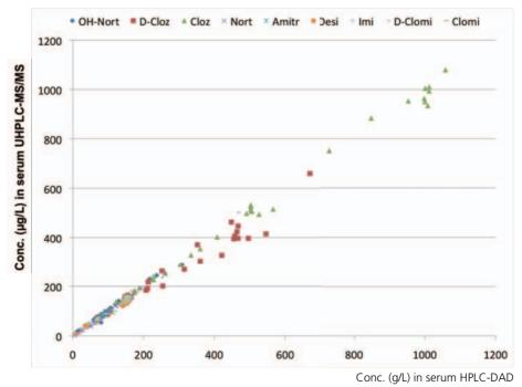
Fig. 3 Comparison of measured results with HPLC-DAD with UHPLC-MS/MS. N-desmethylclozapine shows signs of ion-suppression
