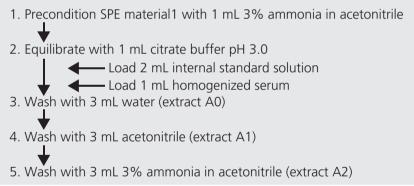
1: Bakerbond Speedisk C18 Polar Plus, 10 µm, 50 mg/3 mL (JT BAKER)
