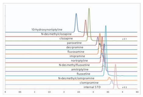
Fig. 2 Mass chromatograms of antidepressants and metabolites in calibration standard (concentration of each compound : 90-100 μg/L in serum, except clozapine: 600 μg/L)
