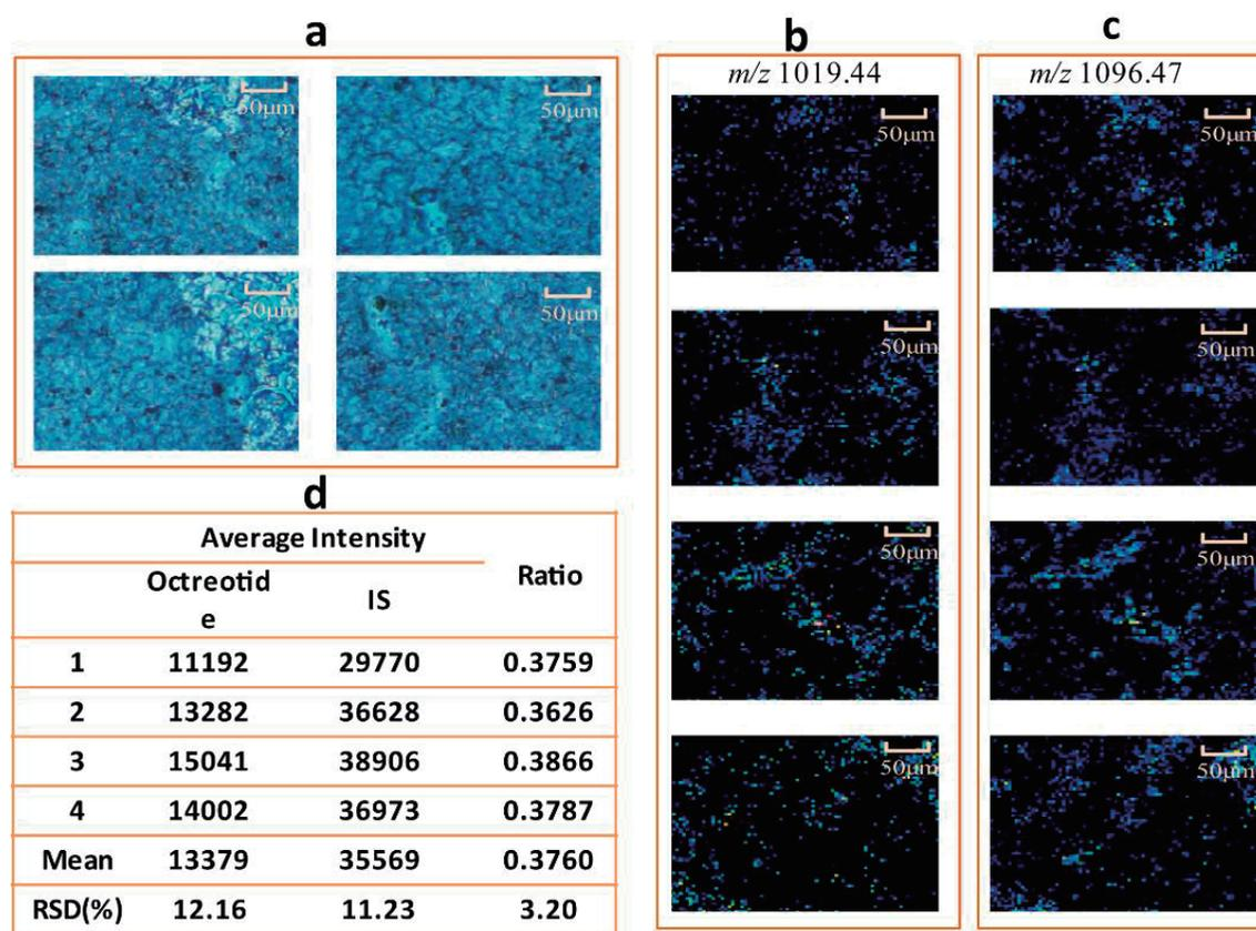
Figure 4 The average intensity ratio of octreotide and IS in four sections of blank stomach tissue covered by the same concentration of the analytes determined based on AP-MALDI-QIT-TOF-iMScope (The scale bar was 50  $\mu$ m).
