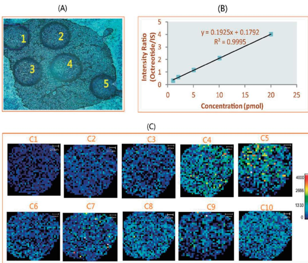
Figure 3 Calibration curves of octreotide constructed by plotting the average intensity ratios (octreotide/lanreotide) against the concentrations in mouse stomach section determined based on LDI-QIT-TOF-IMS (The scale bar was 50  $\mu$ m).
