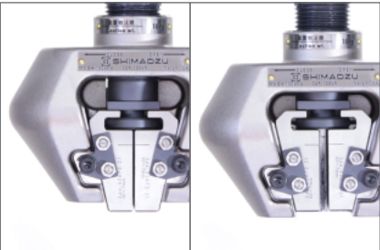
Grip faces stay in the same vertical position when opening and closing
