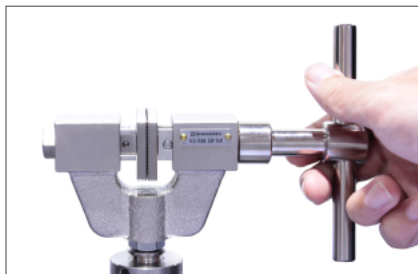
1 kN and 5 kN grips: closed and opened by a T-wrench
