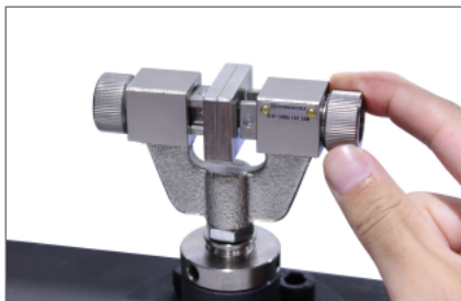
50 N grip: closed and opened by fingers
