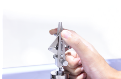
Self-tightening action by spring mechanism
