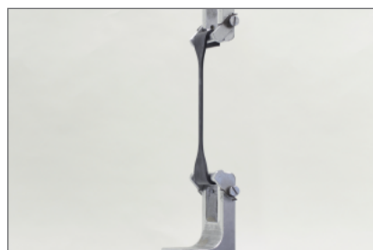
Self-clamping action of upper and lower grips
