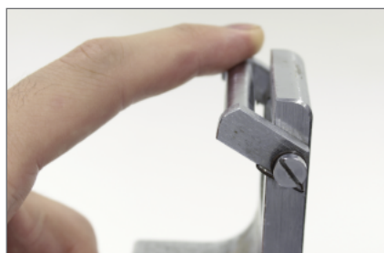
Roller to grip a specimen
