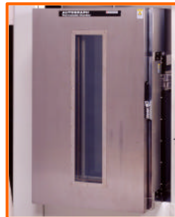
System using thermostatic chamber (Temp. range: -180 to 320°C)
