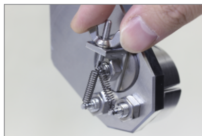
Adjustment screw of gripping force
