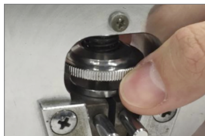
Adjustment screw for gripping force
