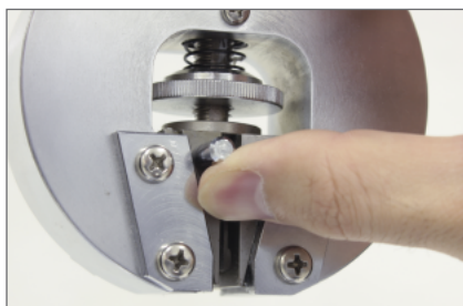
Grips open by raising the attached pins
