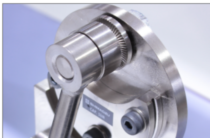
File-teeth grip faces and guide groove
