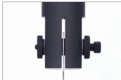
Bushes line the specimen up with the testing axis
