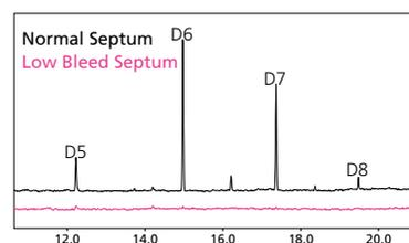
Evaluation by blank analysis, vial heating condition 80 °C
