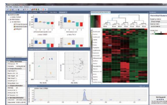
Traverse MS data analysis software is intended for high-speed processing of MRM data acquired with Shimadzu triple quadrupole LCMS systems in the field of targeted metabolomics. Using multiple samples and multiple components, the software is able to create graphical and statistically analysis for metabolic pathway analysis.
