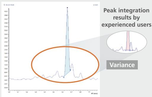
A complicated peak shape due to impurities. Individual differences occur in quantitative results due to correction by manual peak integration.
