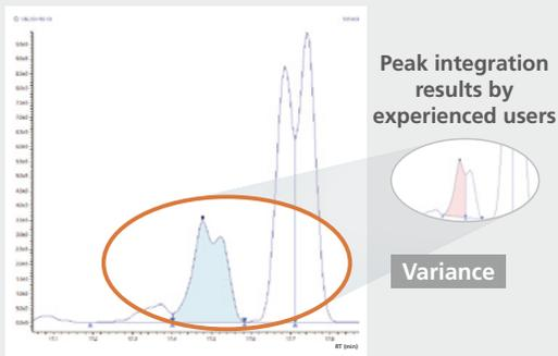
If peaks cannot be separated correctly, corrections via manual peak integration are required.
