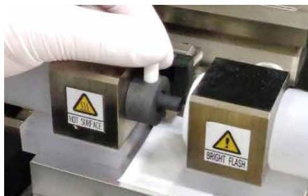
Replacing the Graphite Tube
