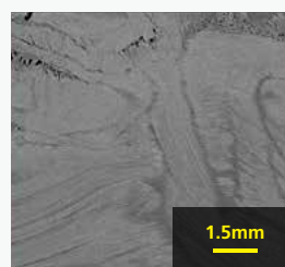
Cross-Sectional Image of the Enlarged Absorption Image of the Area in the Yellow Frame, and the Results of an Orientation Analysis (Image obtained with the inspeXio SMX-225CT FPD HR Plus)
