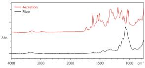
Spectra of contaminants on a textile identified as Phenolic resin
