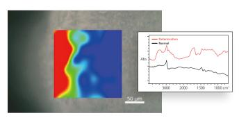
Imaging in the area of the C = O peak indicating oxidation degradation
