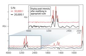
Transmission spectra of 10 µm diameter polystyrene bead obtained by two infrared microscopes with different noise levels.
