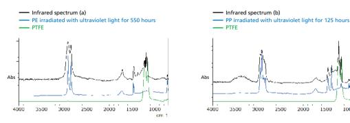
Infrared spectra (a) and (b) extracted from mapping analysis results, and search results
