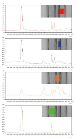
Transmission spectra and chemical image of each layer of multilayer film (First, second, third and fourth layers from the top)
