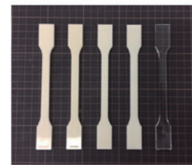
Fig. 1 Sample Appearance Ratios, starting from the left PC:ABS = 0:100, PC:ABS = 25:75, PC:ABS = 50:50, PC:ABS = 75:25, PC:ABS = 100:0
