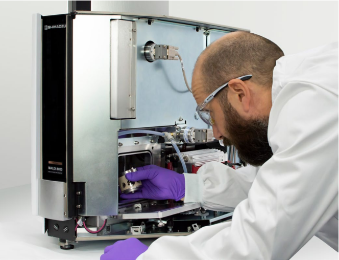
Fig. 4 Designed with the user in mind, the ion optics are easily accessed via a hinged panel following removal of the side cover. Additional safety features built into the instrument design ensure there is no risk of injury from other components during the MALDI EasyCare workflow.
