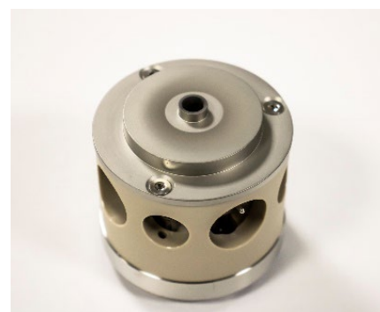
Fig. 2 Contaminated extraction lens. In its normal configuration, the top lens is pointing down towards the sample (see Figure 1). The 'clean' area immediately surrounding the raised boss of the contaminated lens is a result of a shadow effect caused by the boss itself which protects this area from contamination (the white triangles either side of the extended boss in Figure 1).
