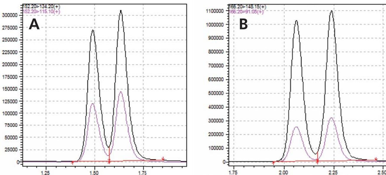
Fig. 2 Chromatograms obtained after an injection of a 5 μL whole blood extract spiked at 200 μg/L.
