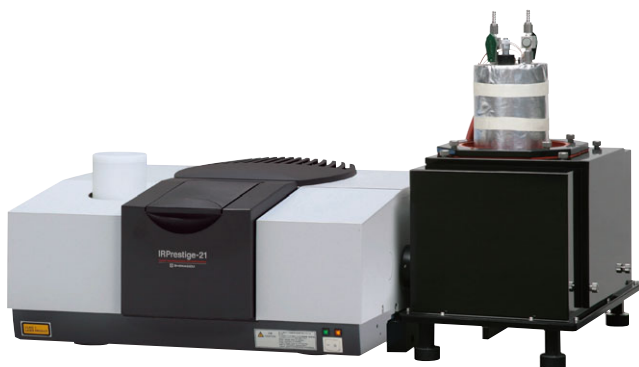
Fig. 4 Gas Cell and Gas Cell Box Positioned Beside the IRPrestige-21
