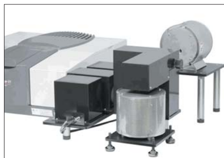
Fig. 2 Appearance of Spectral Emissivity Measurement System
