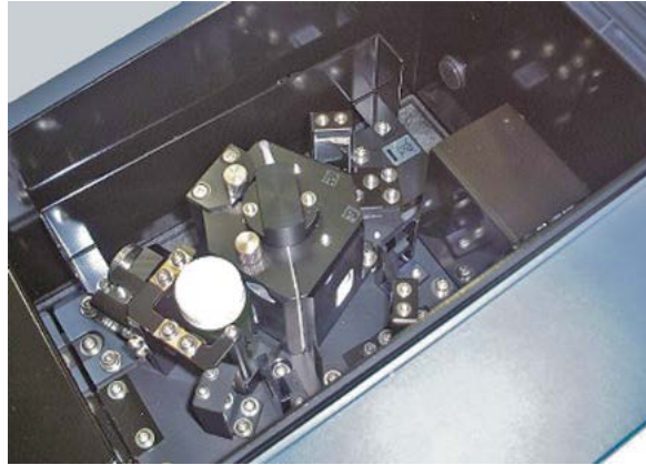
Fig. 2 Integrating Sphere Attachment for Micro Algae Analysis
