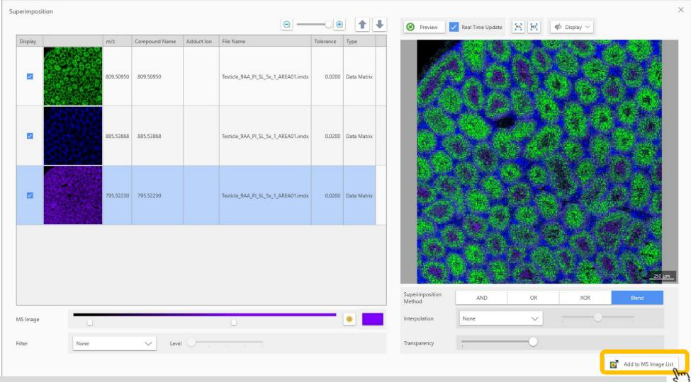
The created superimposition image can be added to the list of MS images on the main screen.
