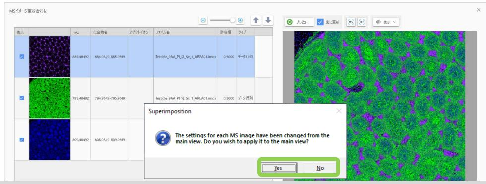
Click "Yes", the colours assigned to each m/z in the superimposed image will be applied to the main window. Click "No", the images in main window will not change.
