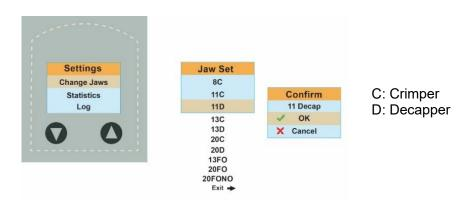
For example, to set the tool to decap 11 mm vials, select Settings Mode >Change Jaw > 11D > Confirm
