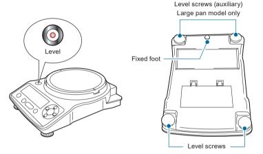
Level the balance by following the procedure below.
