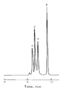
Fig.2 Typical chromatogram of a mixture of proteins on DIOL-150
